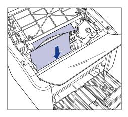
$\ \square$  If the paper is difficult to pull out, pull on the leading edge of the paper as shown in the diagram ①, then remove the paper from the output tray side ②.
